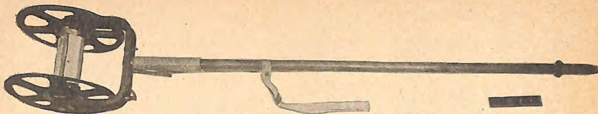
Figure 371. Hand wire reel unit with broomstick handle.
